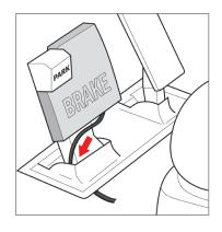
4. Drill (2) small holes in the pedal compartment close to the driver side (red arrow). Secure the LGT-B9 wire out of the way with a cable tie.
